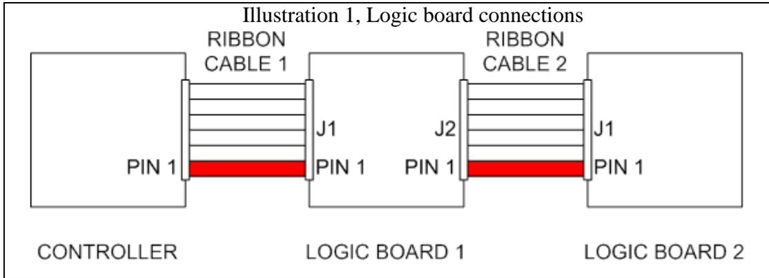
**Note: Attaching the ribbon cable without the red line on pin 1 on each of the headers may cause damage to the controller or the logic board.**
